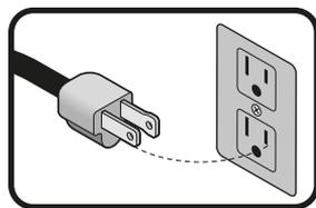
**⚠ WARNING** When using an extension cord, make sure to use a gauge sufficient to carry the current your tool will consume. A lower gauge cable will cause voltage drops in the line, resulting in power loss and motor overheating. The following table shows the correct size to be used depending on the cable length and the amperage capacity indicated on the tool's data plate. If in doubt, use the next higher gauge.
